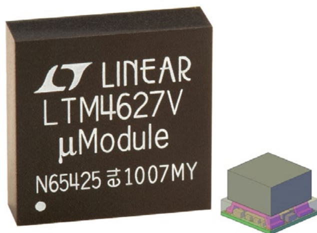
Figure 3. LTM4627 (15 mm × 15 mm × 4.92 mm) vs. its new, smaller equivalent, the LTM4638 (6.25 mm × 6.25 mm × 5.02 mm).
