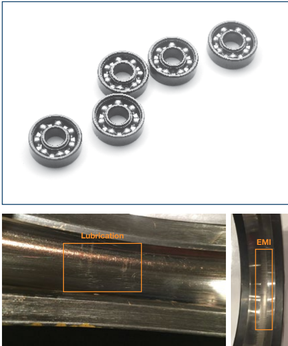
Figure 5. Examples of (top) rolling element bearings and (bottom) lubrication and discharge current defects.
